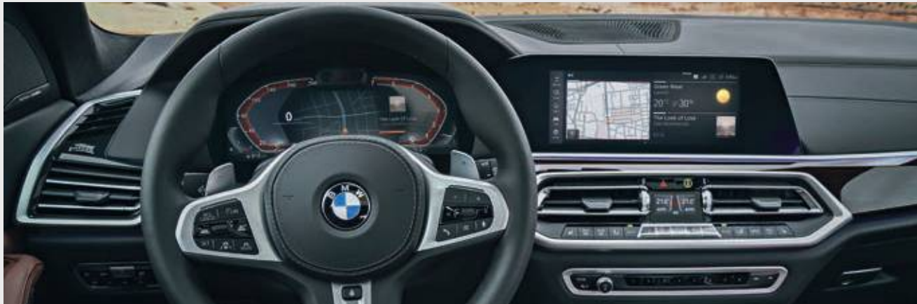
The BMW Live Cockpit Professional with navigation function includes a high-quality display network consisting of a high-resolution 31.2 cm (12.3 inches) Info Display that can be operated by touch and a fully digital 31.2 cm (12.3 inches) instrument cluster.
