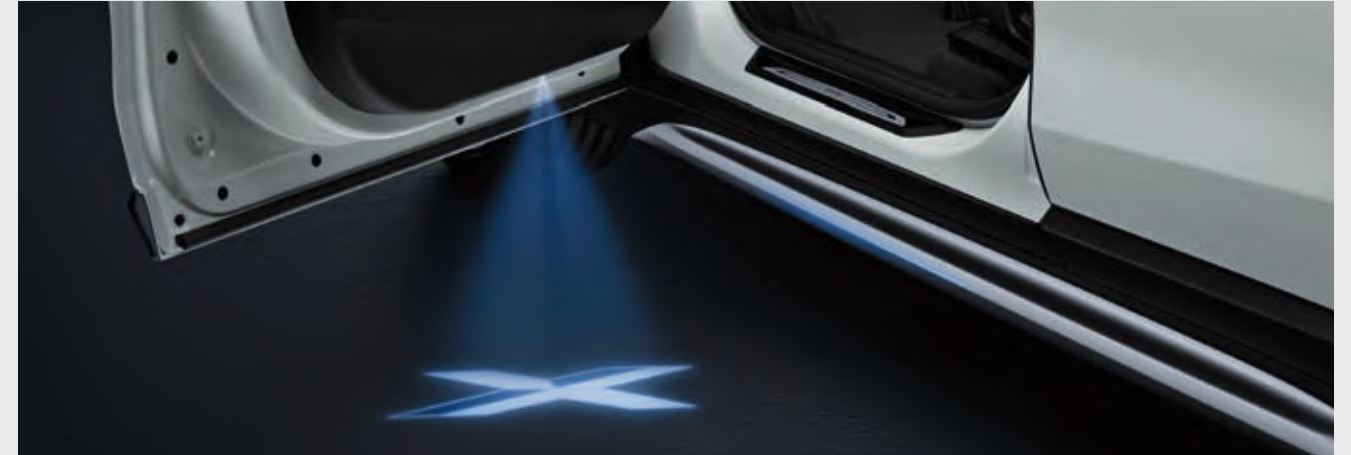
LED Door Projectors. The innovative door projectors are automatically activated when the doors are opened. They project an image onto the ground next to the car using an interchangeable slide.
