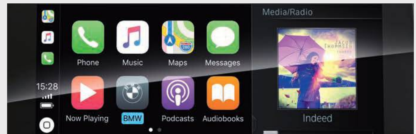
Preparation for Apple CarPlay 1,2 supports the convenient and wireless use of selected iPhone® functions in the vehicle. This allows smartphone content and functions such as music, iMessages/text messages, telephony, Siri and selected third-party apps to be displayed and operated via the vehicle's user interface and via voice control.
