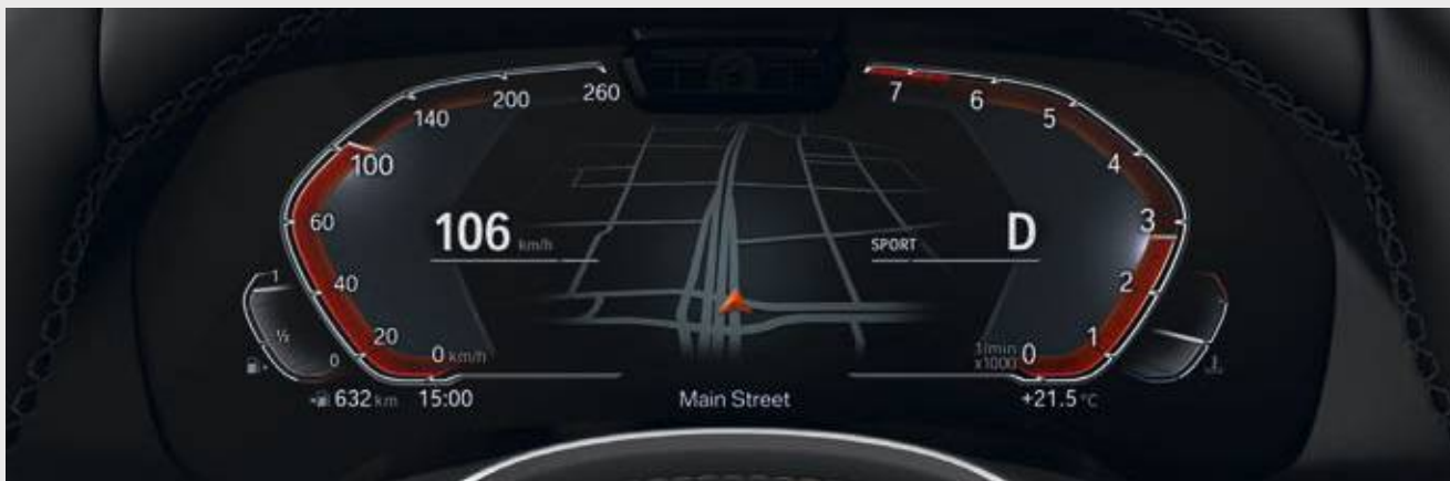
The 31.2 cm (12.3 inches) Multifunctional Instrument Display allows a fully digital display of different content, in addition to speed and revs, including navigation instructions, radio/multimedia track lists and phone lists.
