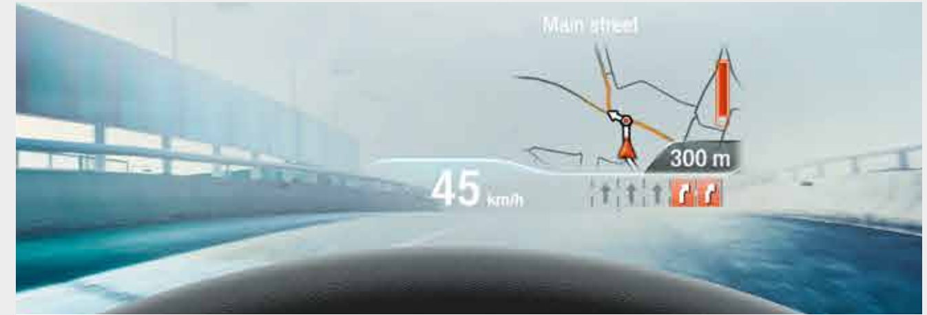
BMW Head-Up Display offers a full-colour projection of driving relevant and situational information onto the windscreen with improved resolution of 800 x 400 pixels.
